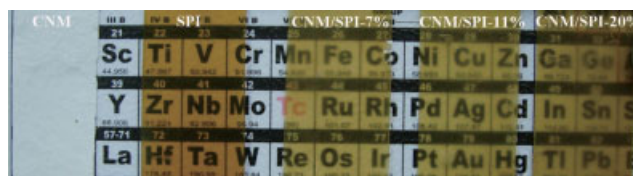
Figure 4 Appearance of CNM, SPI, CNM/SPI composite films placed on a periodical table. The percent value is CNM content in the composite. [Color figure can be viewed in the online issue, which is available at www.interscience.wiley.com .]
